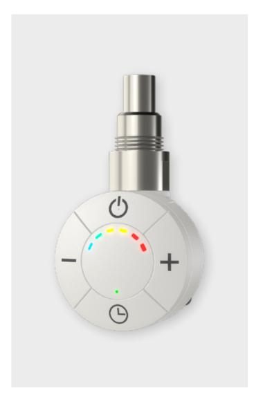
Electronic thermostat for electric towel heaters based on fluid heat transfer. The **ambient** temperature is controlled by means of an external sensor. The **SMART** series has the heating element couples to the thermostat. The symmetry of the device enables both right and left side coupling to the towel heater. It is possible to choose between three predefined programs, as indicated in the guide for setting the operational times.
