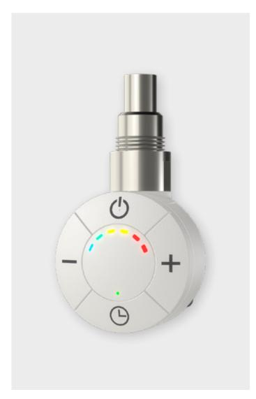
Electronic thermostat for electric towel heaters based on fluid heat transfer. The temperature is controlled by means of an internal sensor. The **SMART** series has the heating element attached to the thermostat. The symmetry of the device enables both right and left side coupling to the towel heater. It is possible to choose between three predefined programs, as indicated in the guide for setting the operational times.
