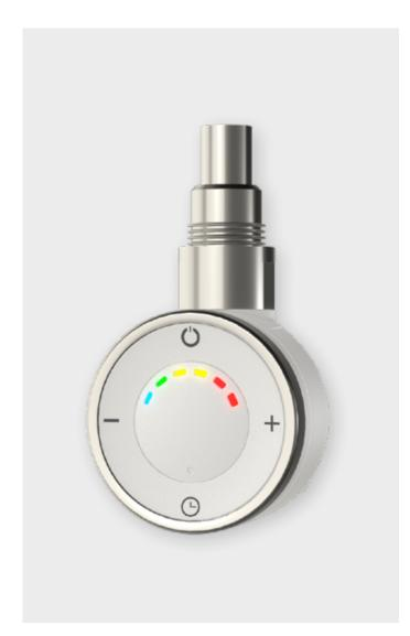
Electronic thermostat for electric towel heaters based on fluid heat transfer. The temperature is controlled by means of an internal sensor. The **EVO** series has the heating element attached to the thermostat. The symmetry of the device enables both right and left side coupling to the towel heater. It is possible to choose between three predefined programs, as indicated in the guide for setting the operational times.
