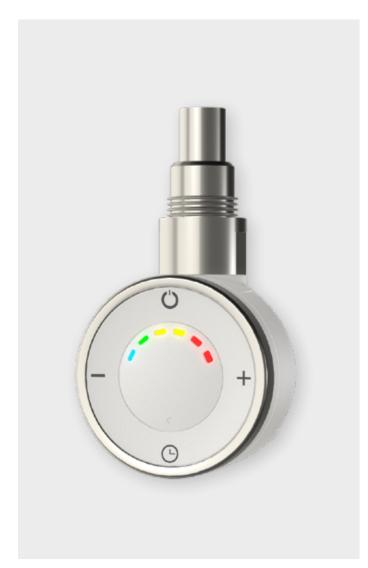
Electronic thermostat for electric towel heaters based on fluid heat transfer. The **ambient** temperature is controlled by means of an external sensor. The **EVO PLUS** series has the heating element couples to the thermostat. The symmetry of the device enables both right and left side coupling to the towel heater. It is possible to choose between three predefined programs, as indicated in the guide for setting the operational times.
